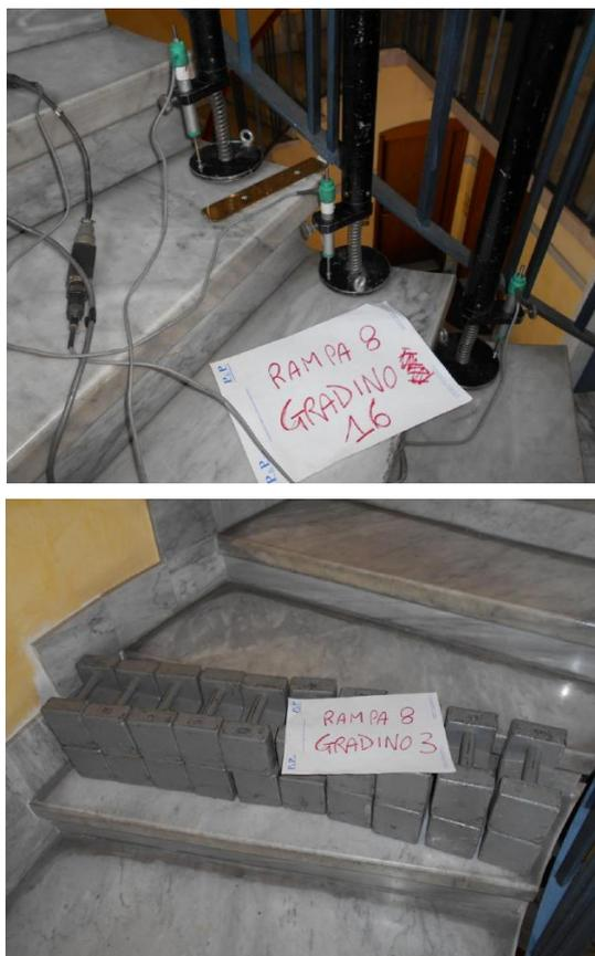
Fig. 10. Instruments adopted for load tests
