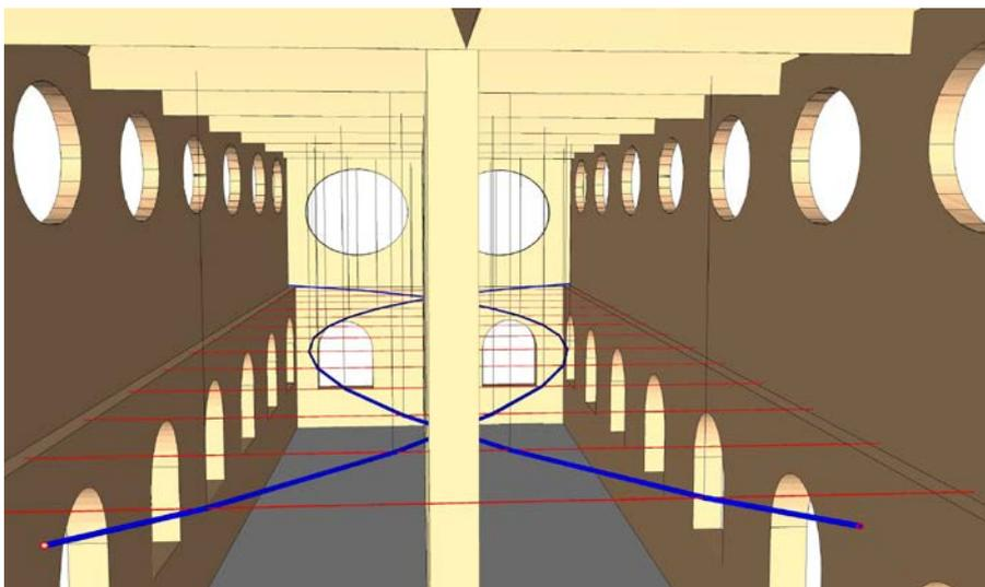
Fig. 6. Bracing of the building at an intermediate level of the big room.
