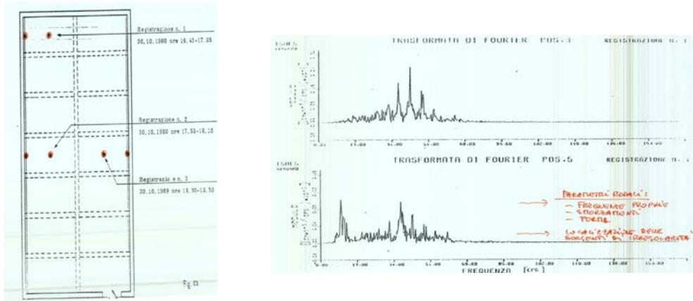
Fig. 2. Dynamic tests recorded on Palazzo della Ragione (1980). Plan view with the position of the accelerometers and accelerogram of two points after application of the Fast Fourier Transform (FFT)
